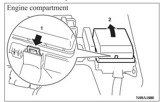
In the engine compartment, the fuse block is located as shown in the illustration.
